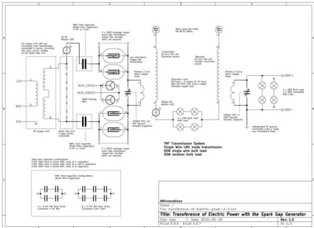
Figure 2 below show the schematic for the transference of electric power experiment powered by the SGG. The high-resolution version can be viewed by clicking [here](#).
